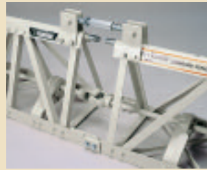
Extended Turnbuckles allow screed to be inverted 1/2 in/ft (12.7 mm/m) versus the normal 1/4 in (6.35 mm).
